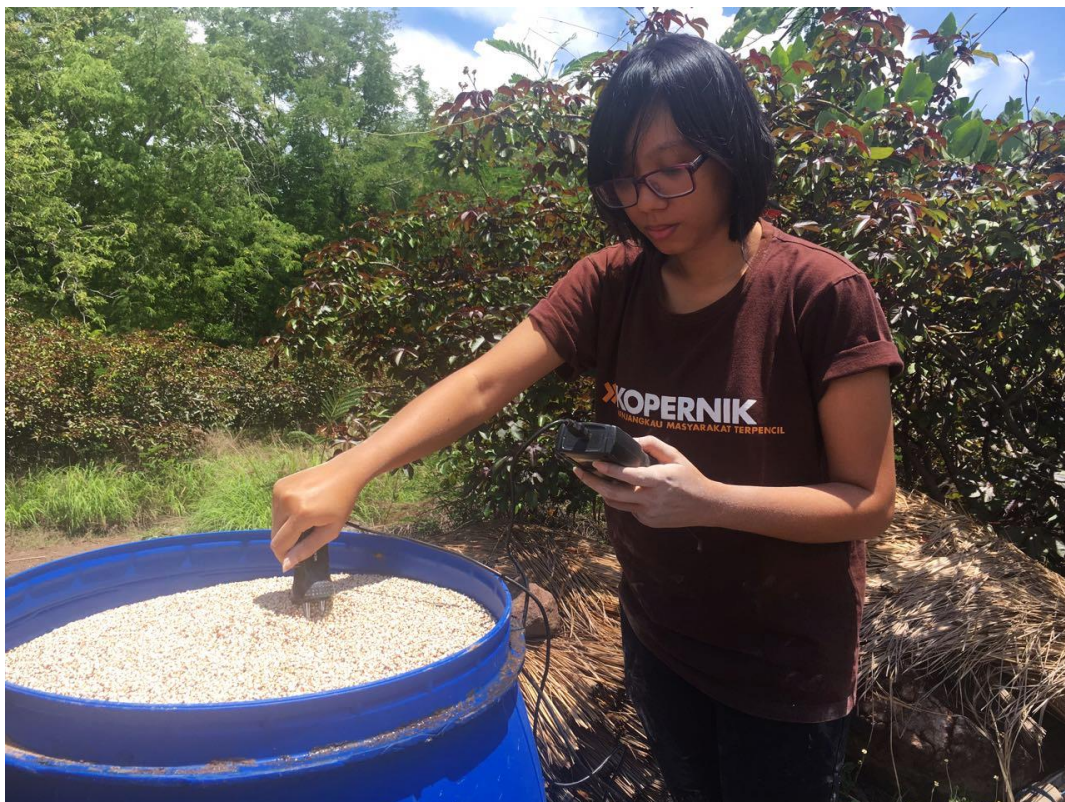
Image 3. A Kopernik Senior Analyst measuring the moisture level of the stored sorghum using a moisture meter
