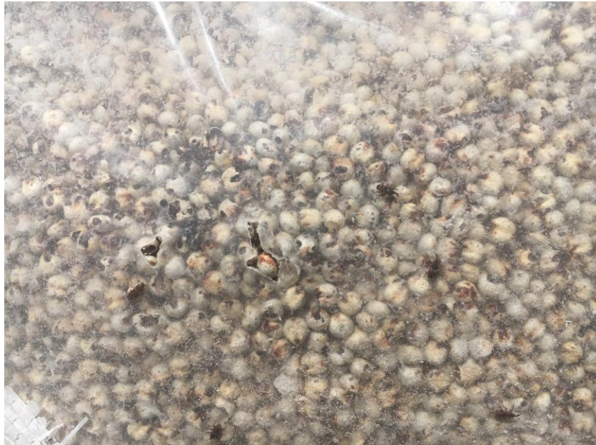
Image 2. Holes were observed on the surface of the hermetic plastic bag, breaching the hermetic seal.
