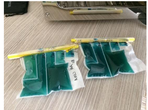
Figure 4. Sample water containing E. coli changes its colour after 40 hours
