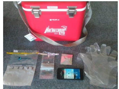
Figure 3. Akvo Caddisfly E. coli test kit (cooler box is optional)
