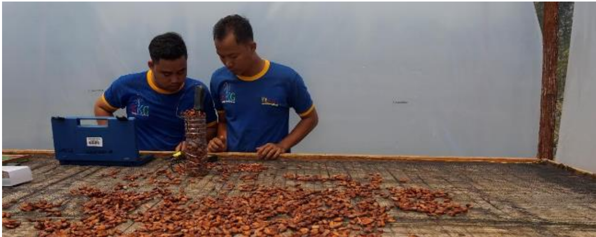
Test of moisture content of the cacao beans being dried.
