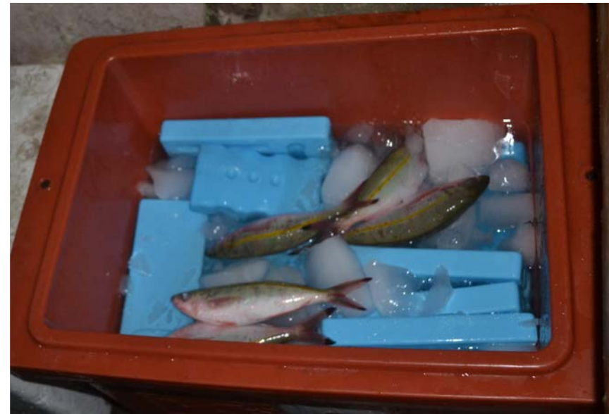
Treatment 3 (cooling solution) Insulated box + ice gel packs
